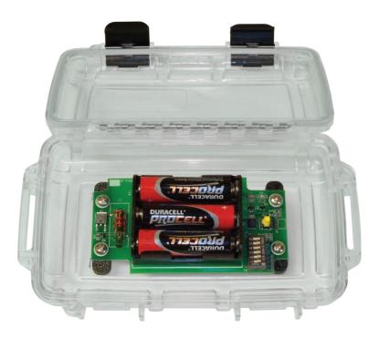
The Marker Tag is mounted within an Otter 2000 enclosure that can be immersed to 100 feet.
