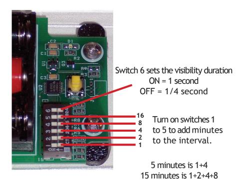
When all switches are off the reader is in a special test mode that reveals the tag every 3 seconds.
