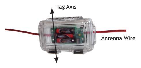
The tag could also be mounted in the read zone at the minimum required distance. The tag axis should point towards the middle of the loop.
